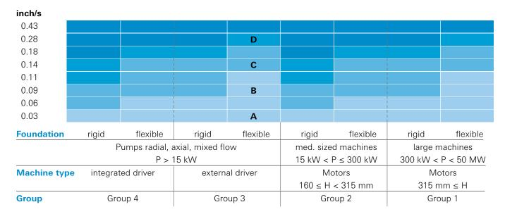
**DIN ISO 10816:** Mechanical vibrations – assessment of the vibrations of machine through measurements on no rotating parts. **Vibration velocity (rms)** 10 – 1000 Hz, n > 600 min<sup>-1</sup>, 2 – 1000 Hz, n > 120 min<sup>-1</sup>
